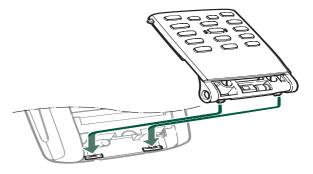
**Note** At the end of the flip key pad there is a hinge, which is adjustable in three positions. Make sure the hinge is in its middle position when you attach it.
