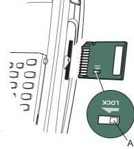
**Note** Insert the Memory Stick Duo correctly to avoid damages to your P800 or the Memory Stick Duo.
